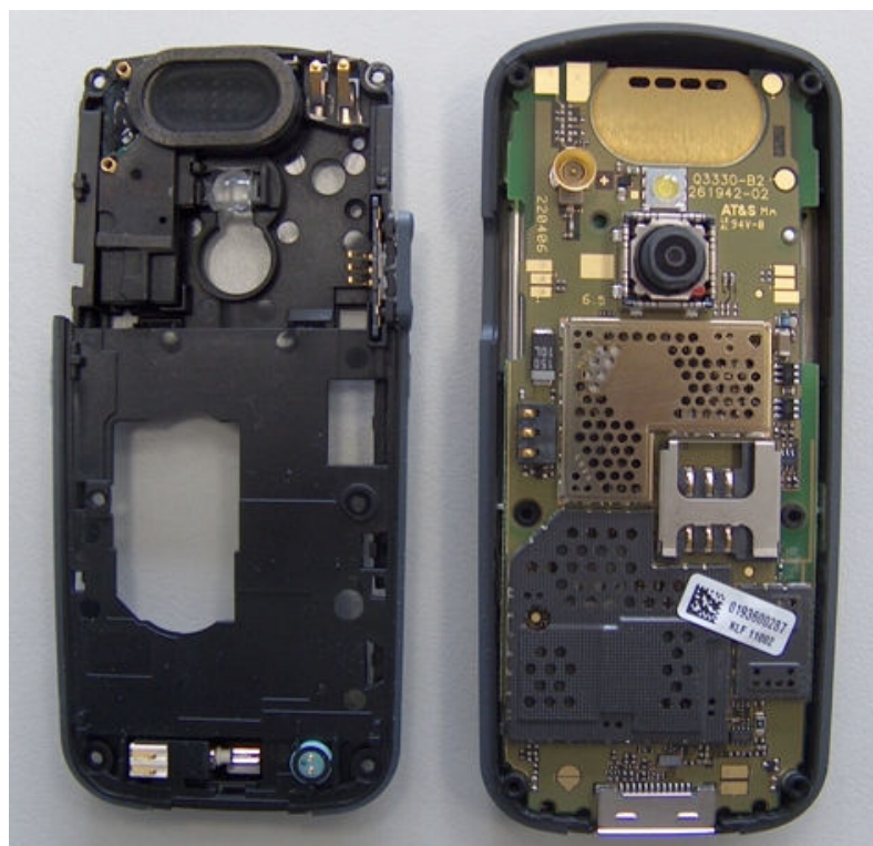
Disassemble Step 1: Lower Case opened
