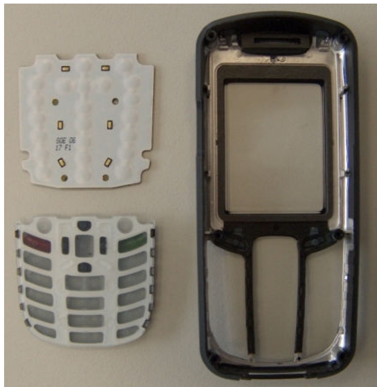
Disassemble Step 3: Front Cover disassembled
