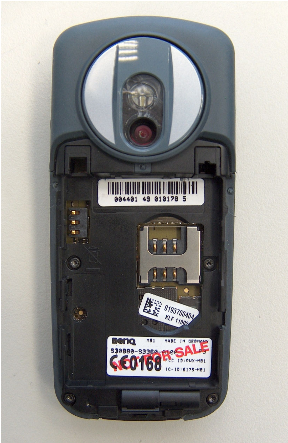
Figure 2 FCC ID and IC ID label placed in M81 from BenQ-Siemens
