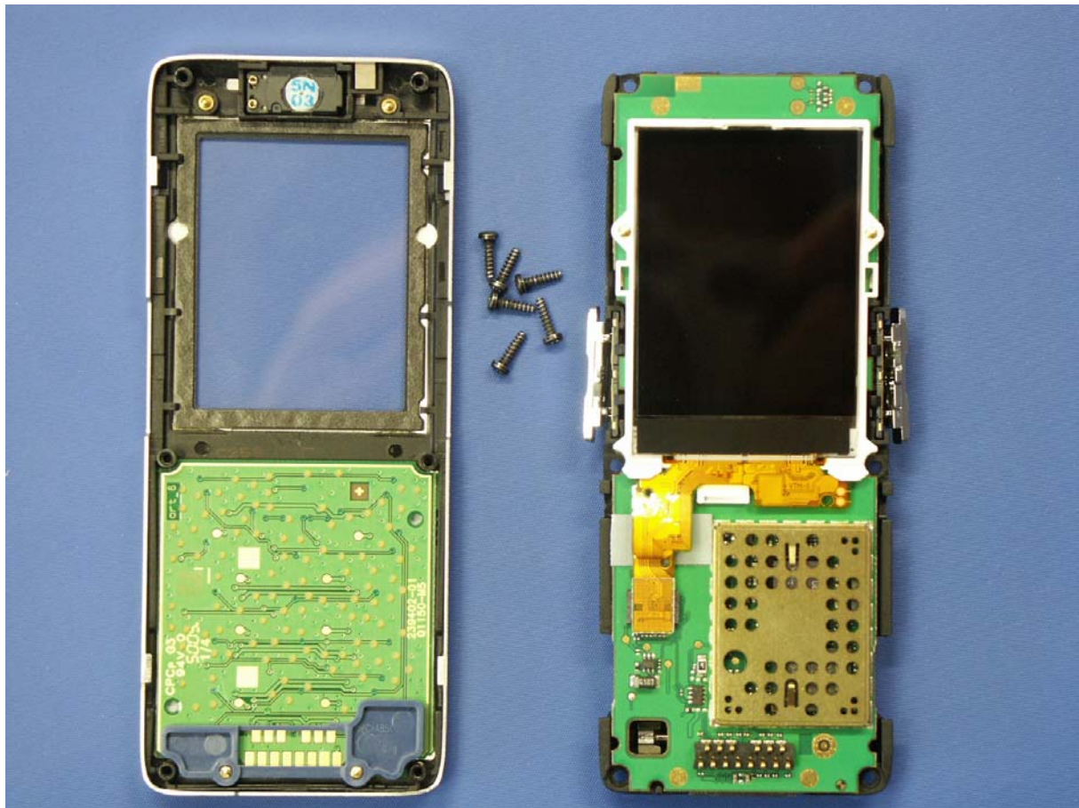
S68 PCB removed
