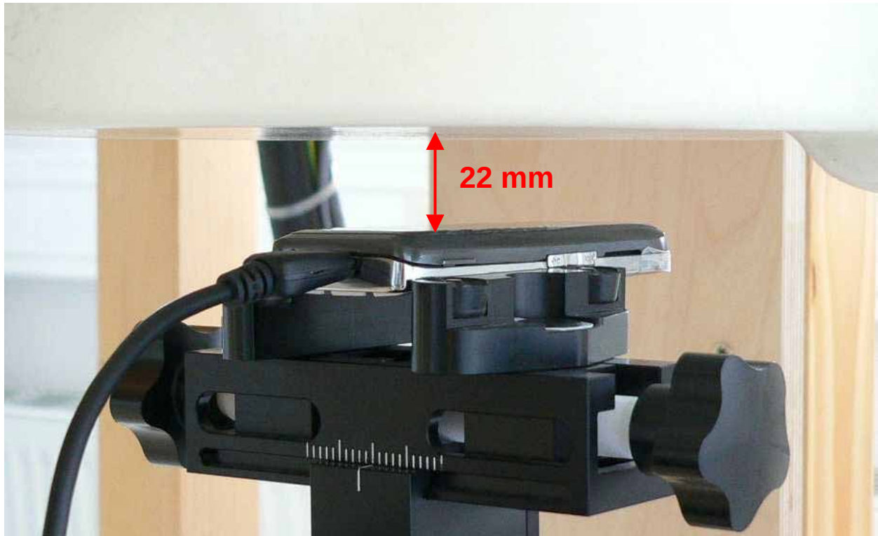
Fig. 27: Body worn configuration BenQ Siemens S68, GPRS (Class 10) mode with data cable, antenna towards the phantom, gap = 22 mm.
