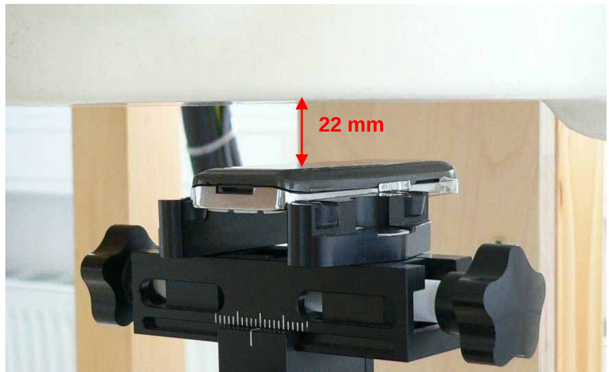
Fig. 28: Body worn configuration BenQ Siemens S68, GPRS (Class 10) mode without accessory, BT activated, antenna towards the phantom, gap = 22 mm.
