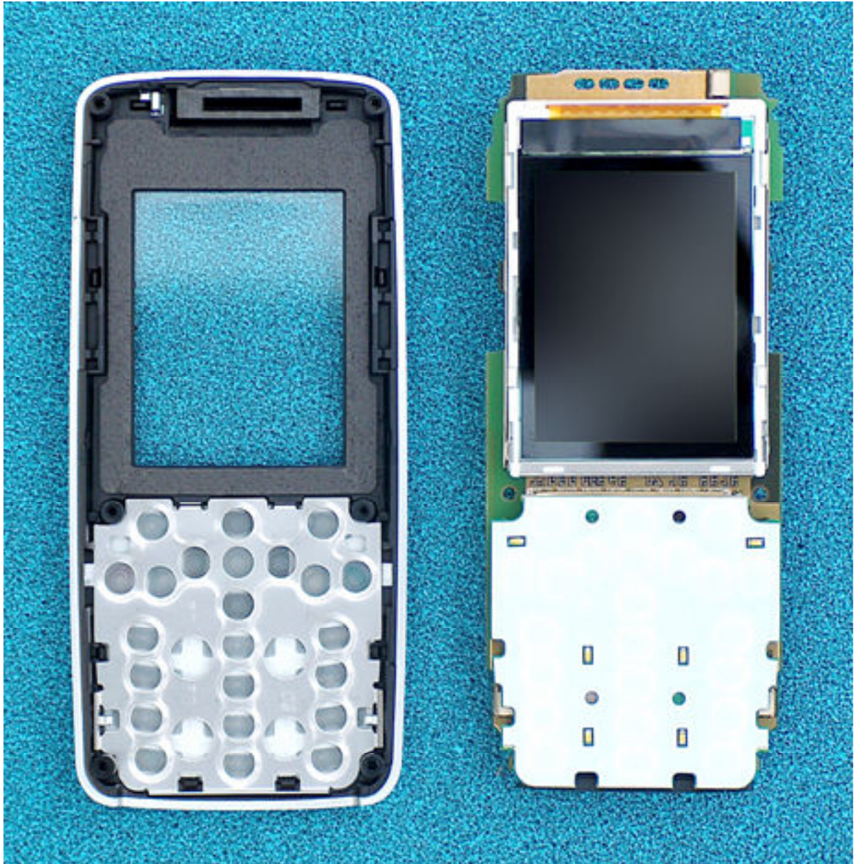
S75 Keypad & Front Cover Disassembly Step 1
