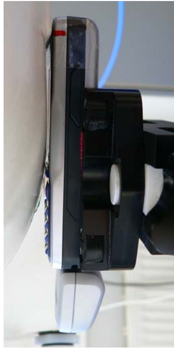
Fig. 28: Cheek position, left side, with flash.
