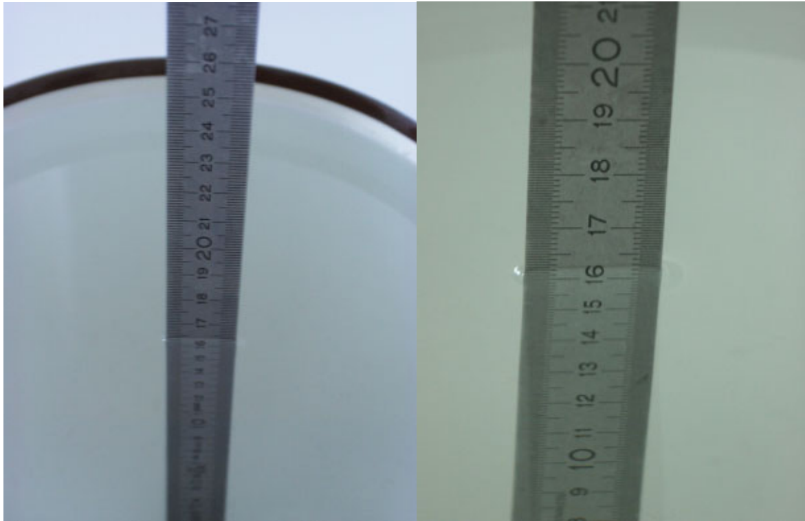
Fig. 24: Liquid depth for PCS 1900 Head and Body measurements.
