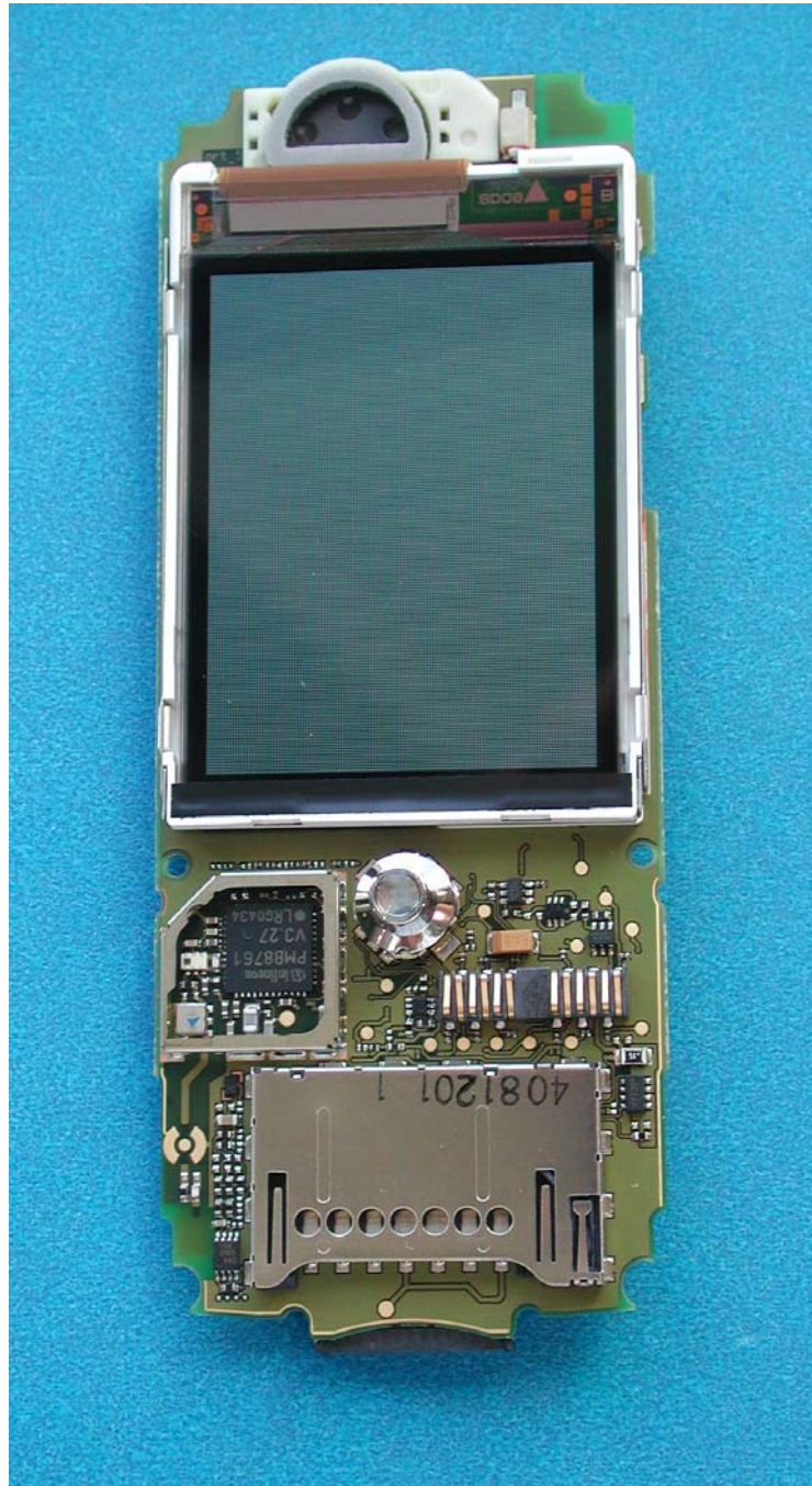
SP65 PCB Front View Shields Removed
