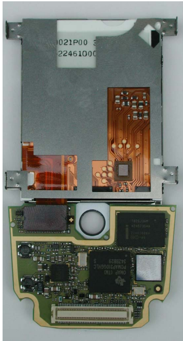
SX1 Auxiliary Board with Keypad & Display (Side 2)
