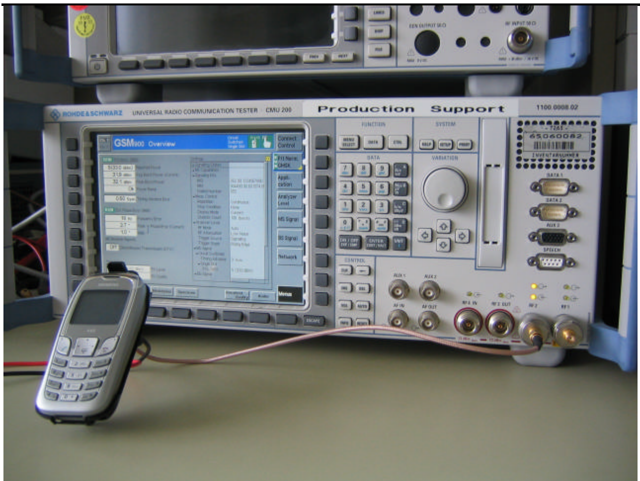
Figure 2: Set-up for conducted power measurement
