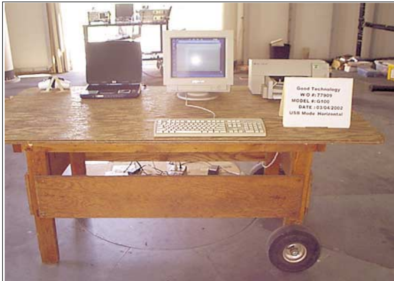
Radiated Emissions - Front View - USB Horizontal
