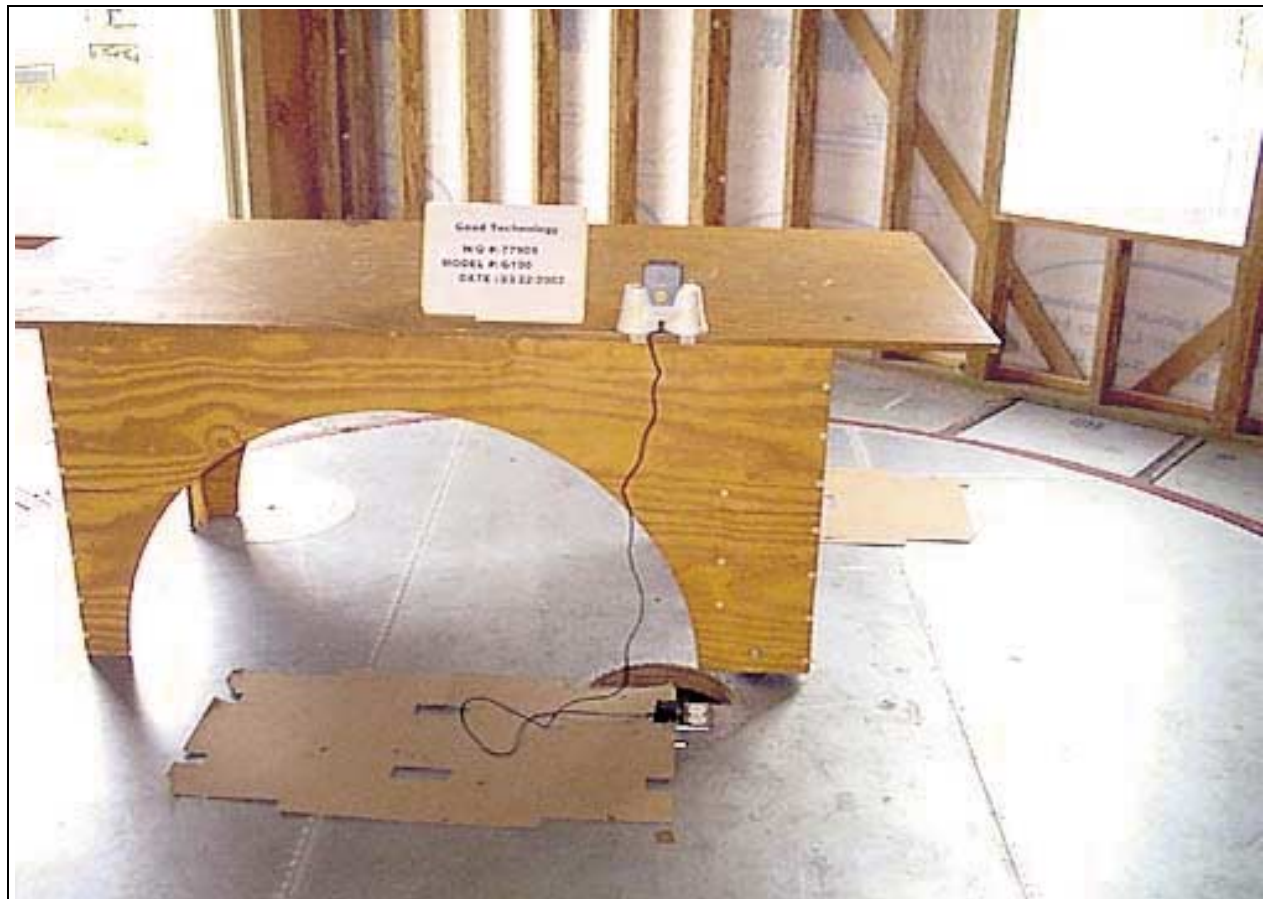
Radiated Emissions - Back View - AC Adapter Vertical
