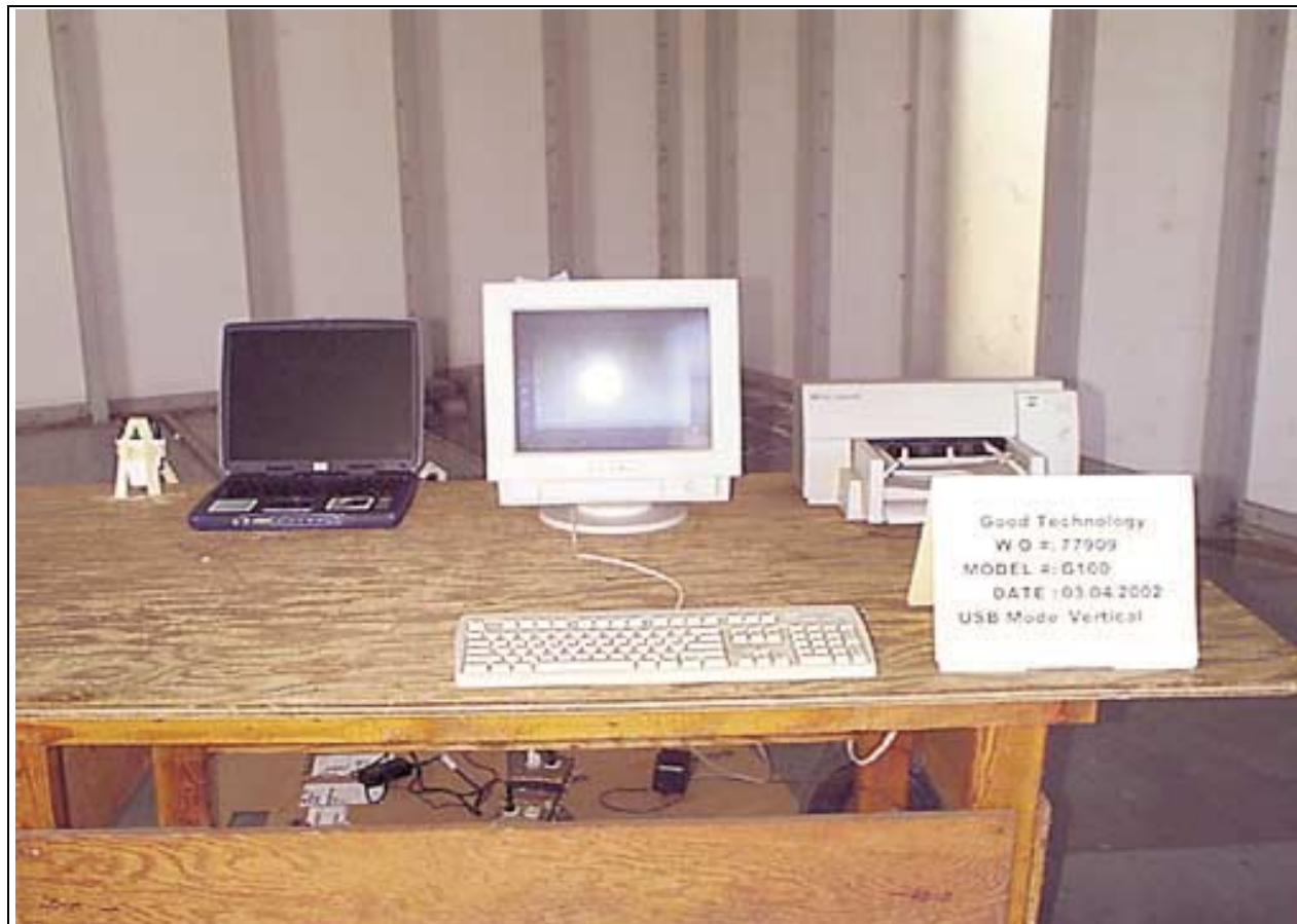
Radiated Emissions - Front View - USB Vertical
