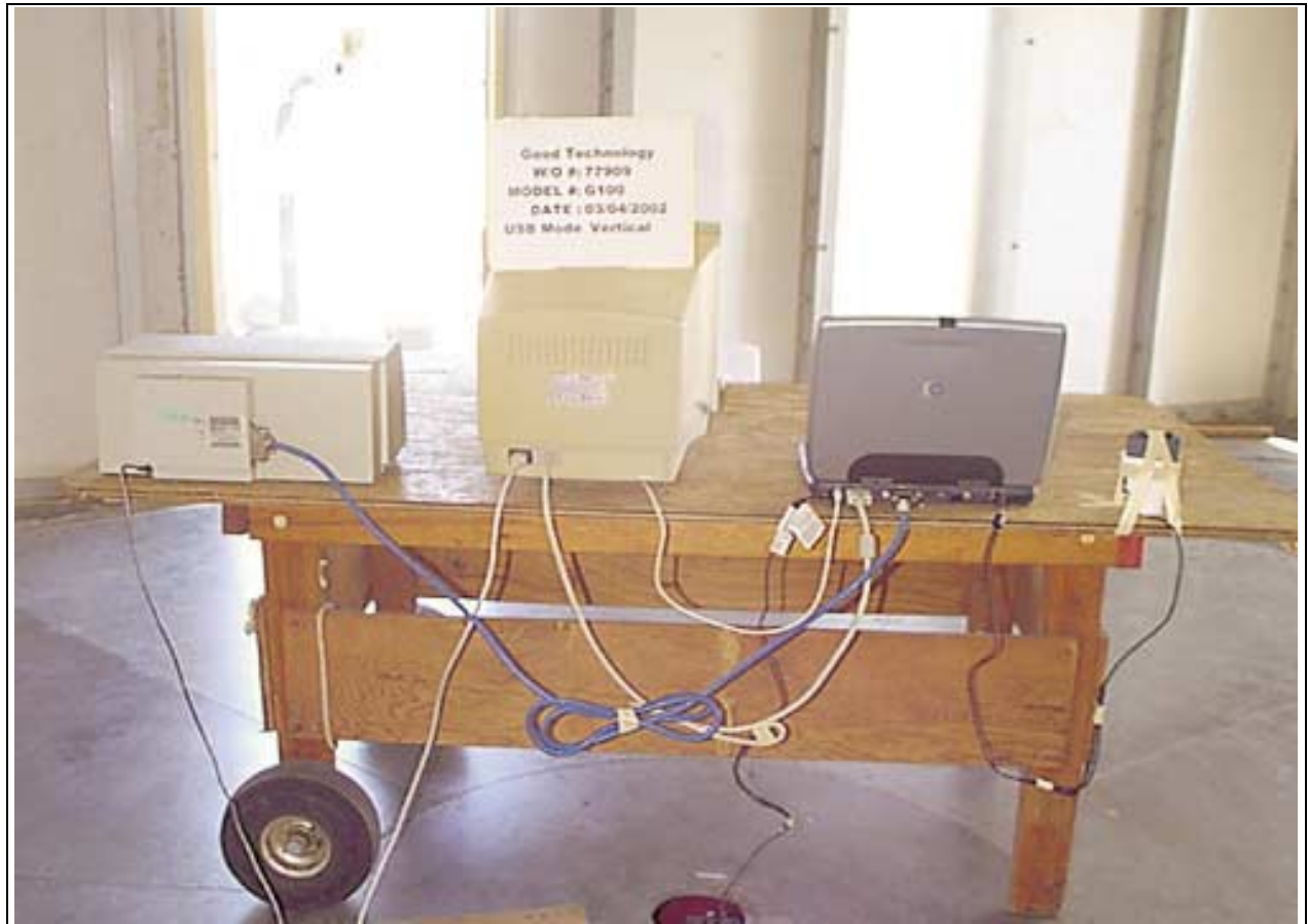
Radiated Emissions - Back View - USB Vertical
