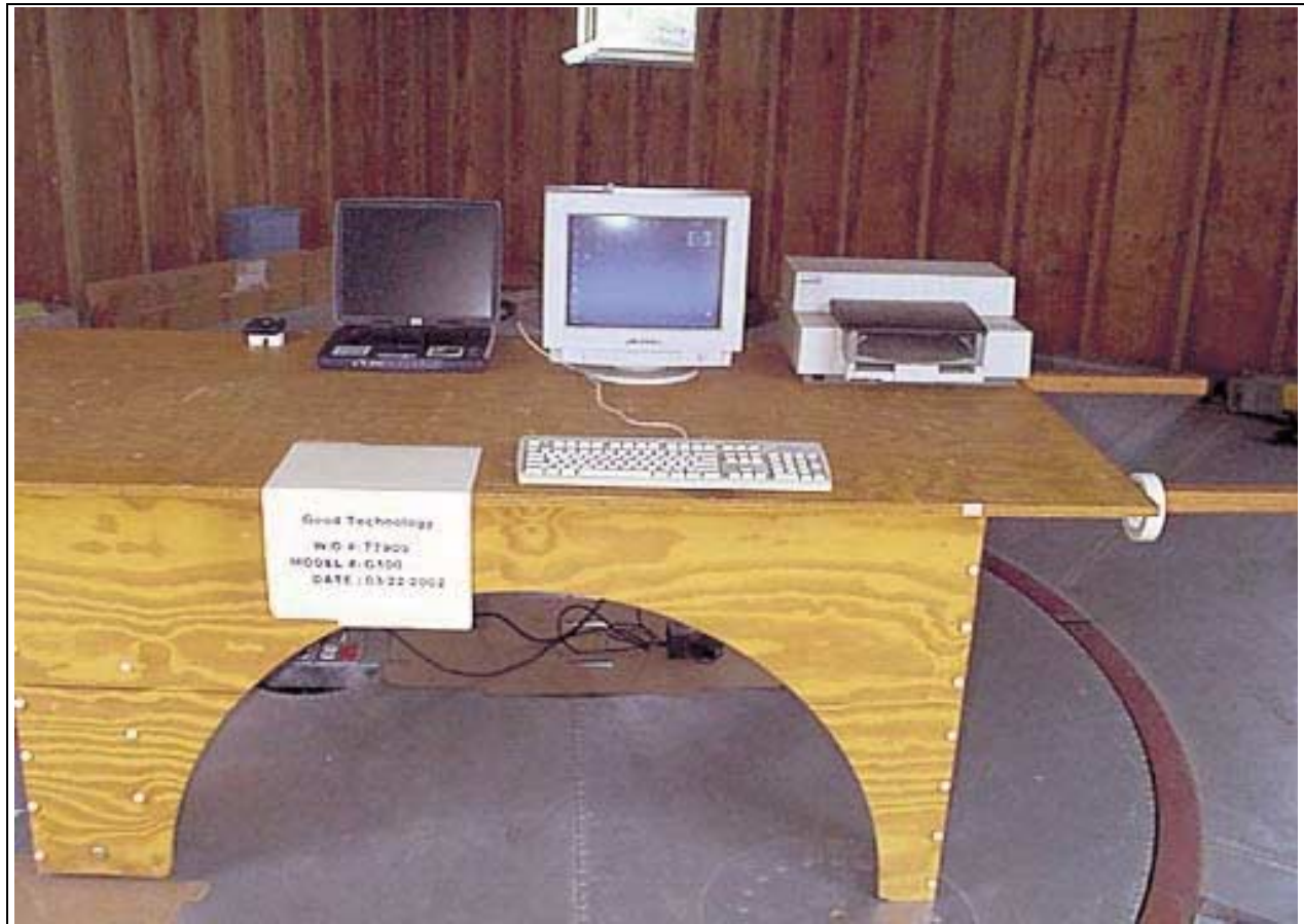
Radiated Emissions - Front View - USB Flat
