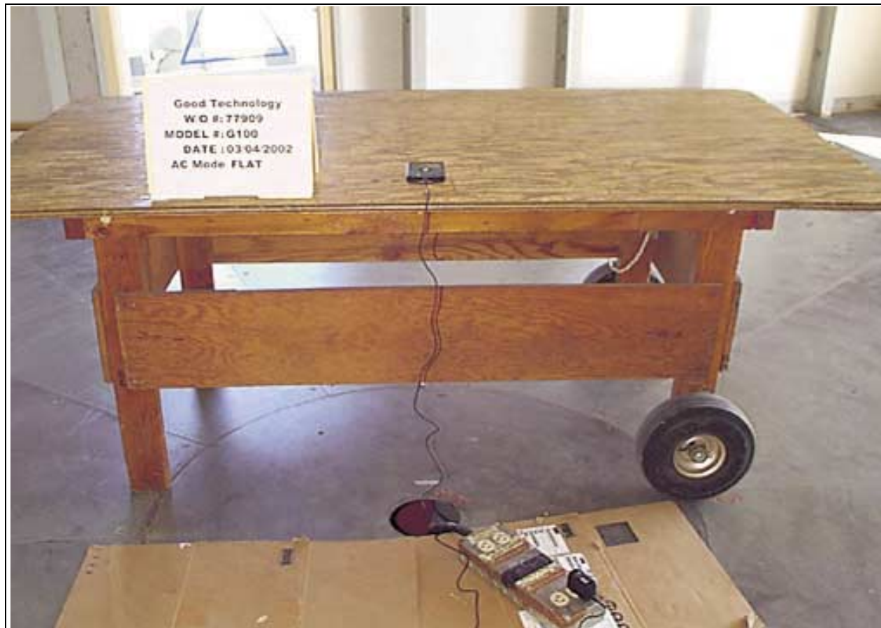
Radiated Emissions - Back View - AC Adapter Flat
