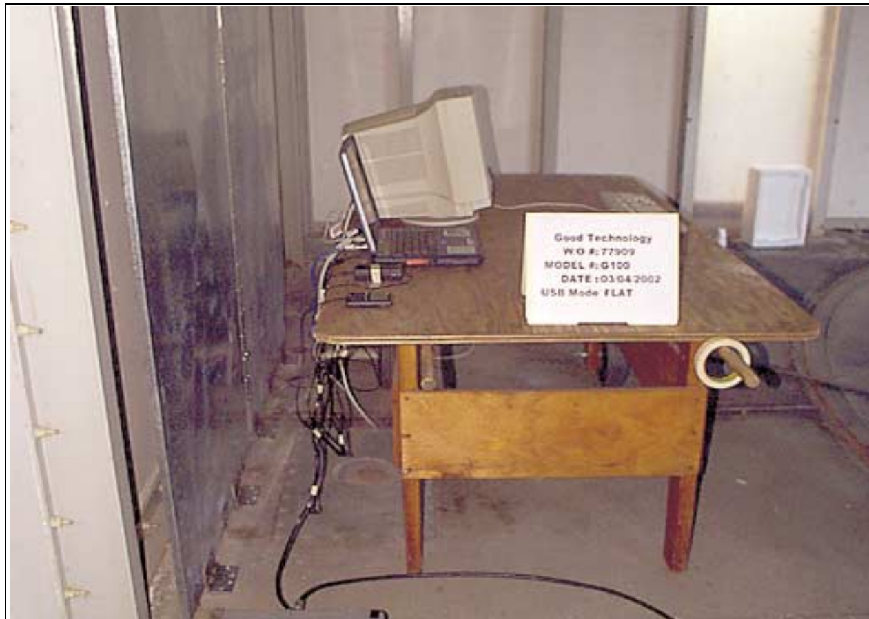
Mains Conducted Emissions - Side View - USB
