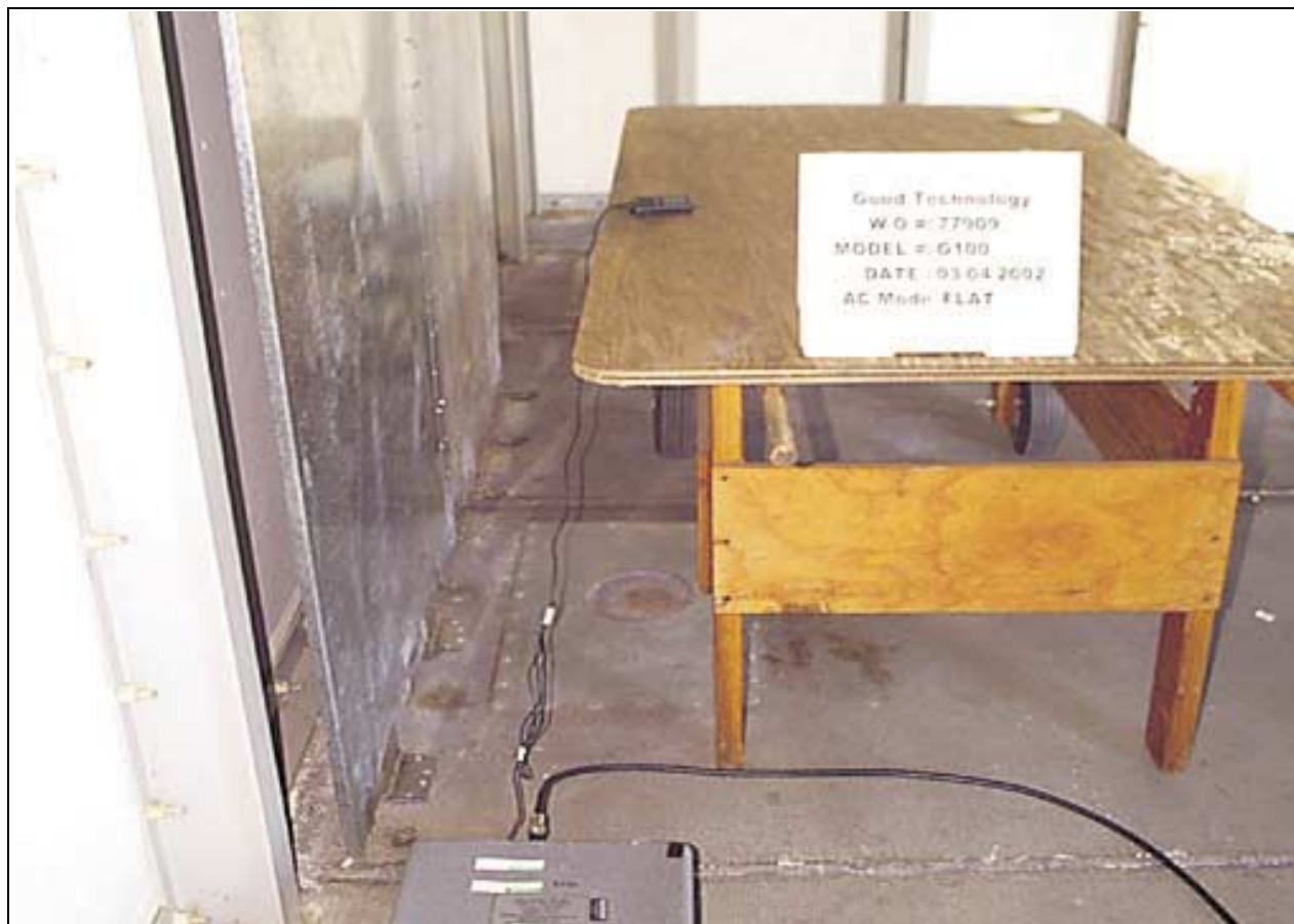
Mains Conducted Emissions - Side View - AC Adapter
