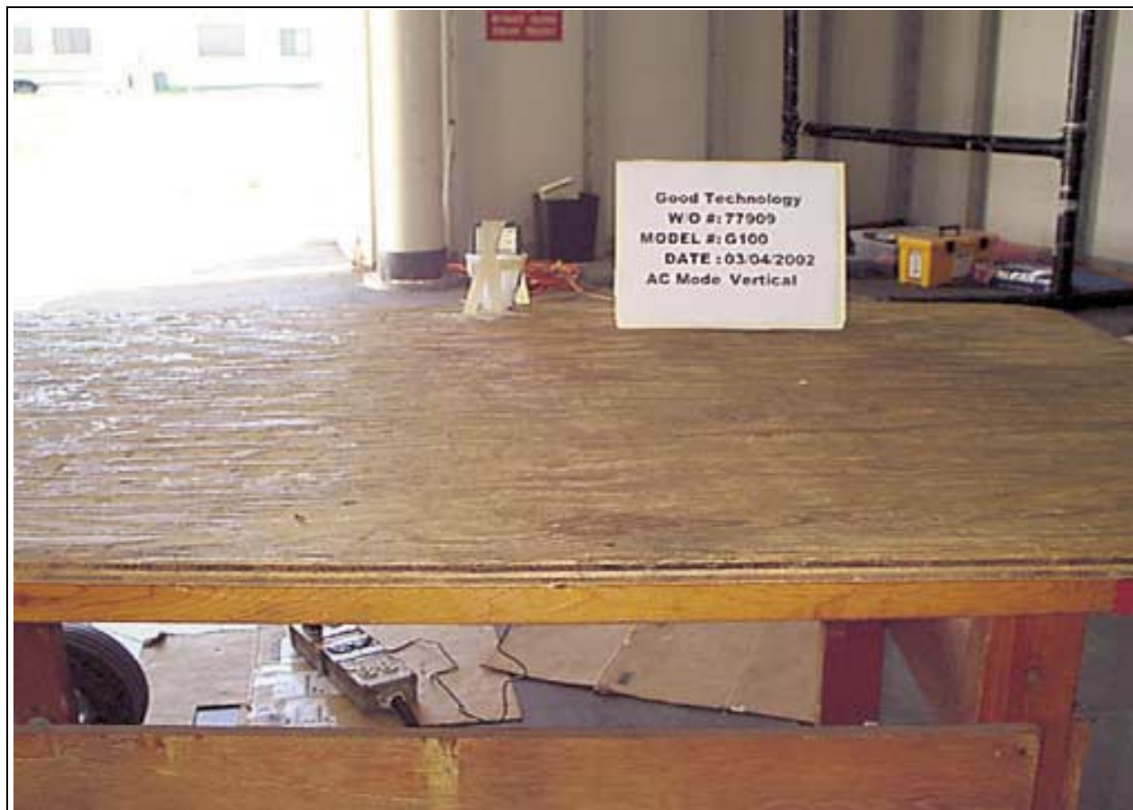
Radiated Emissions - Front View - AC Adapter Vertical
