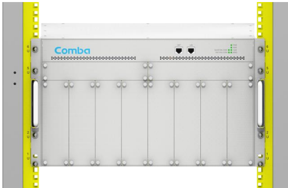
Figure 5: Install cabinet nuts and support screws
