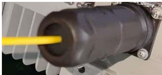
Figure19 Tighten the waterproof cover
