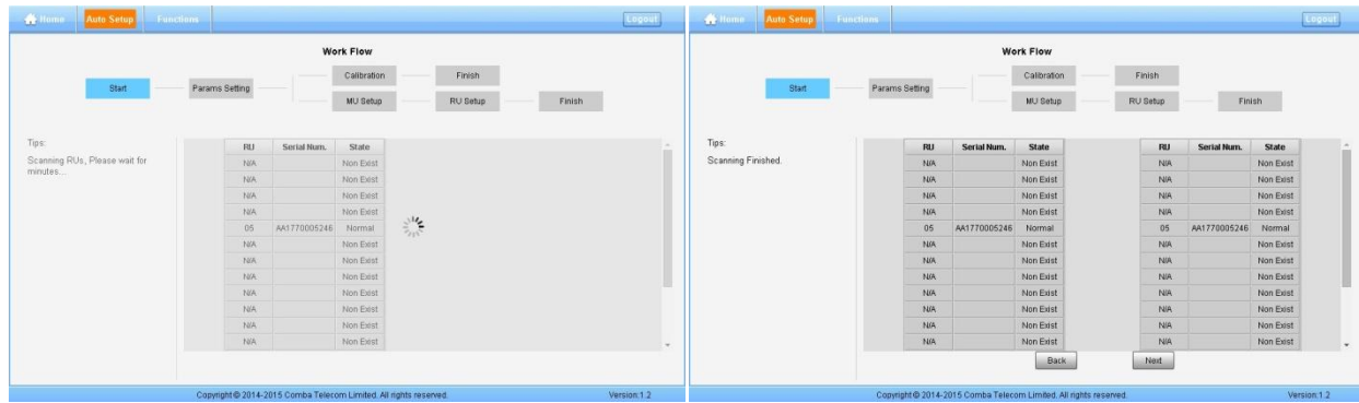
Figure 65: Commissioning Procedure - Device Scan
