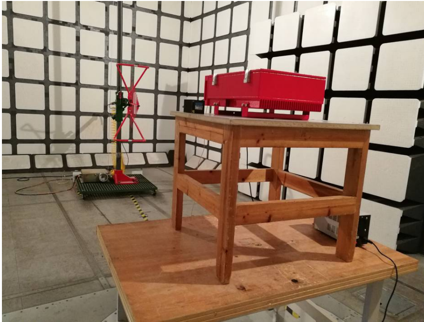
Transmitting Radiated Emissions Tested - Front View (Below 1 GHz)
