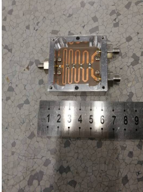
EUT – Splitter Module 2 Board View
