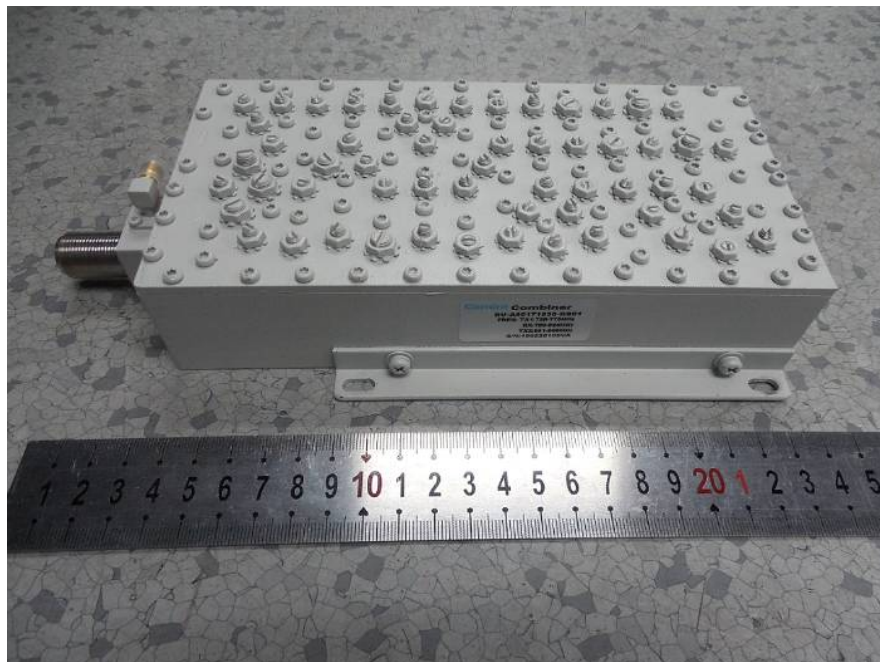
EUT – Duplexer Module View 1
