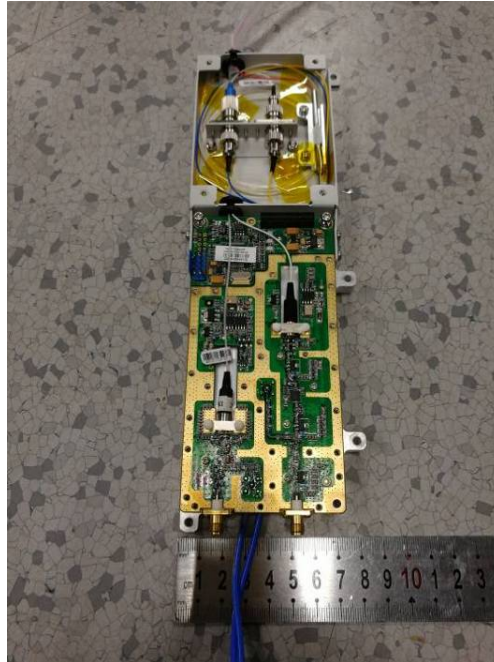
EUT – Optical Module Cover off View
