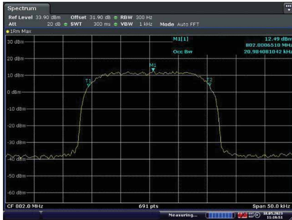
Middle Frequency: 802.0MHz, Output occupied BW(AGC)
