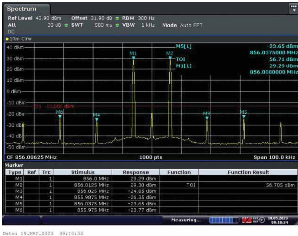
Mid Frequency and with the ALC threshold level
