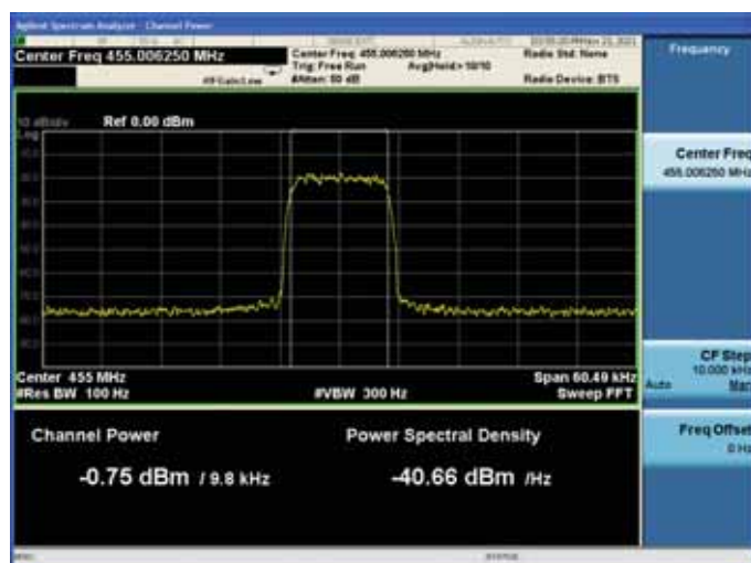
Input signal Low Frequency: 455.00625MHz
