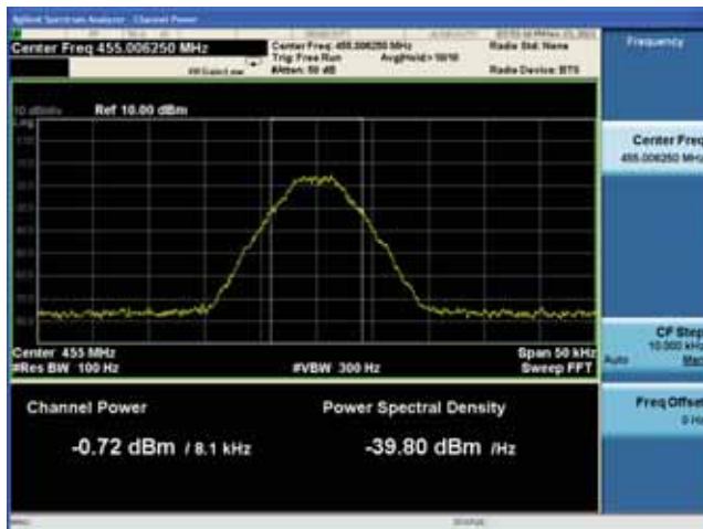
Input signal Low Frequency: 455.00625MHz
