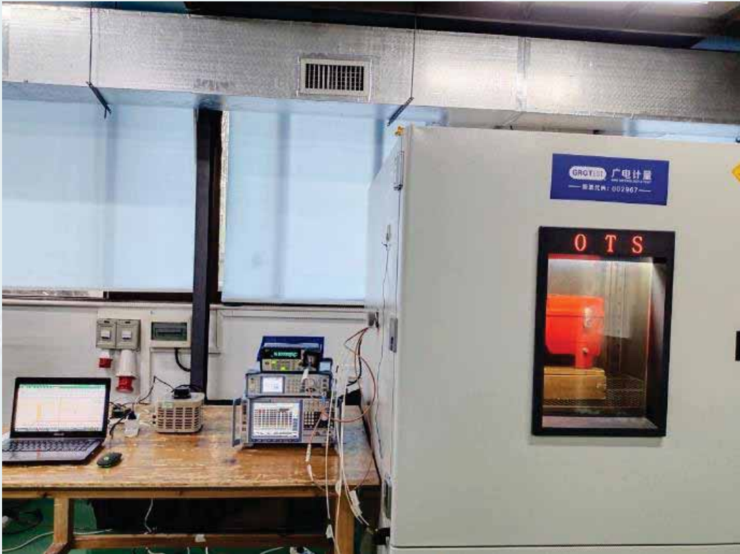
Temperature change test-2
