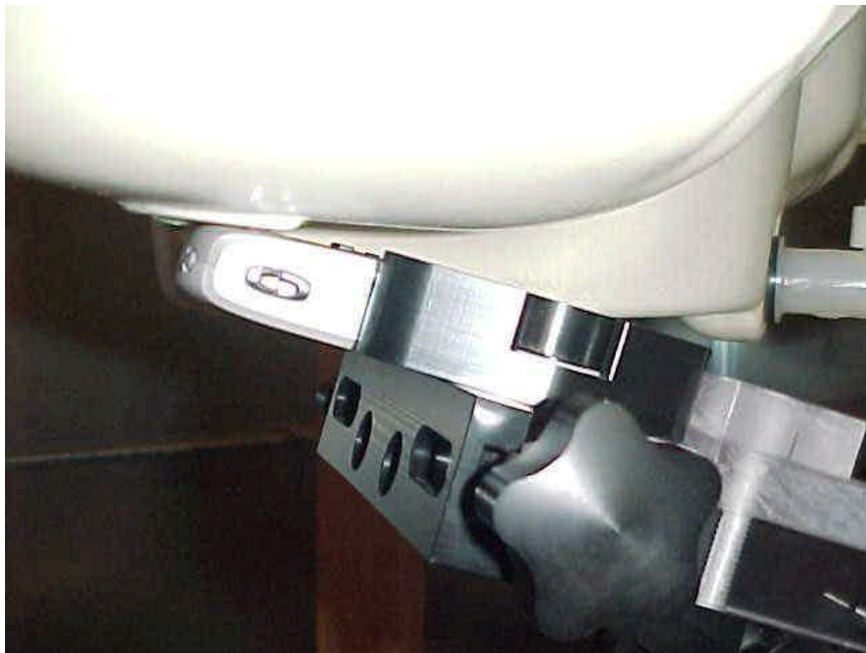
Position of device against head phantom using the “tilt” position
