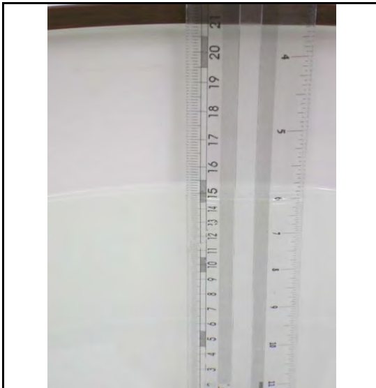
Figure 6. Liquid Height for Body SAR
