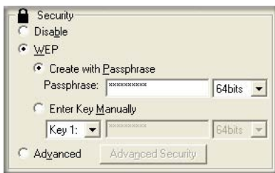
Figure 4-6: WEP Encryption Security
