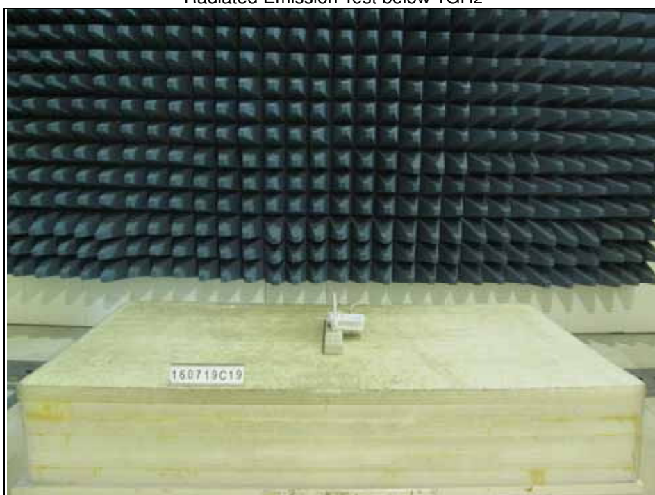
Radiated Emission Test below 1GHz
