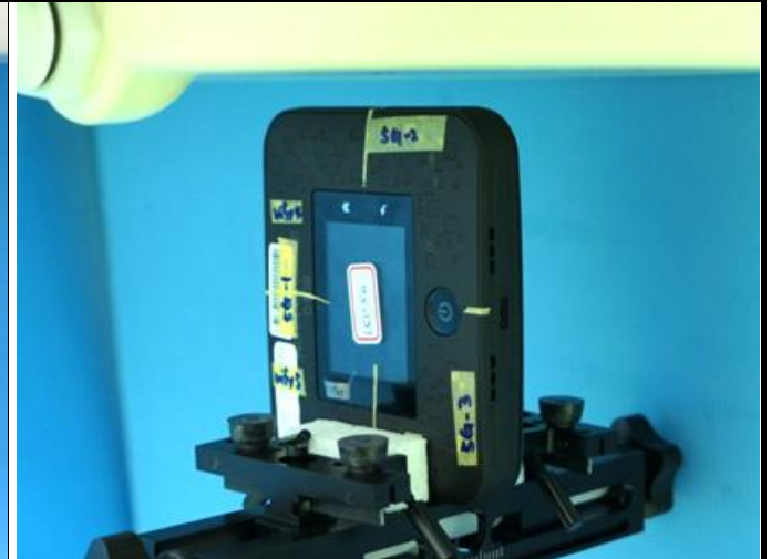
Body - Right Side of EUT at 10 mm
