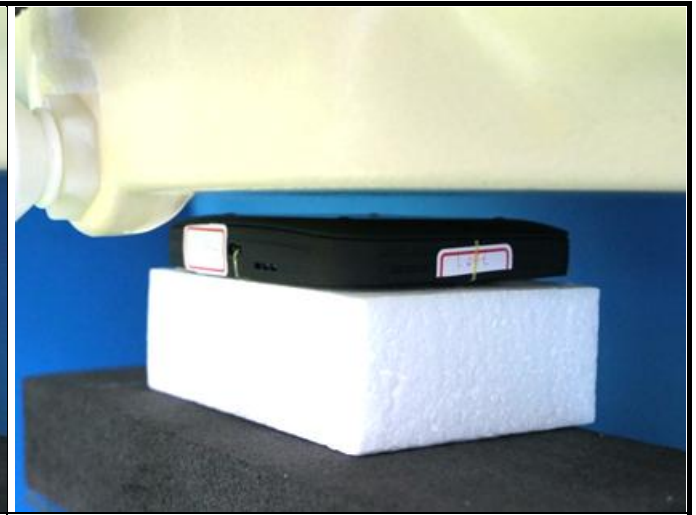
Body - Rear Face of EUT at 10 mm
