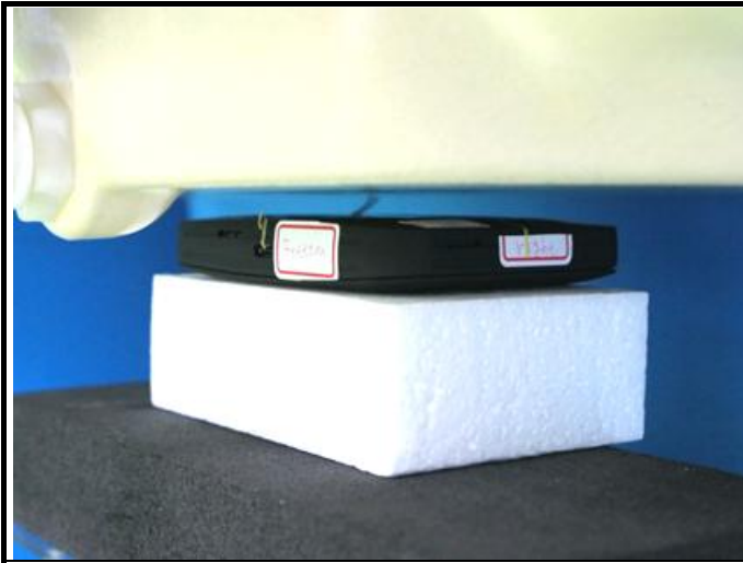
Body - Front Face of EUT at 10 mm
