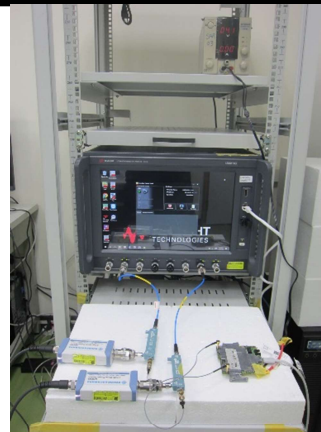
Setup for Conducted Power Test (for ENDC)
