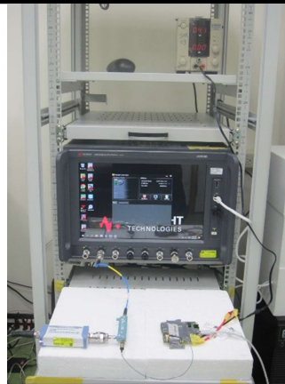
Setup for Conducted Power Test (for 5GNR SA)
