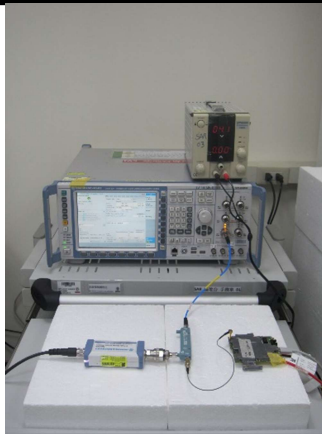
Setup for Conducted Power Test (for LTE band)
