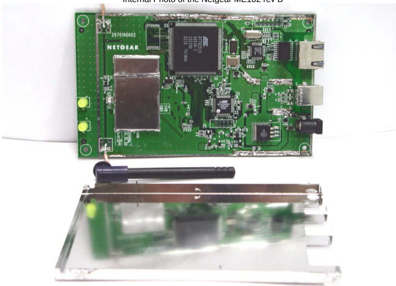
Internal Photo of the Netgear ME102 rev B
