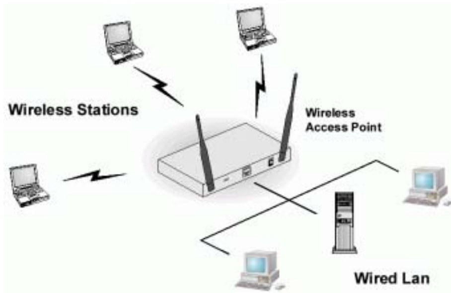
Figure 1: Wireless Access Point
