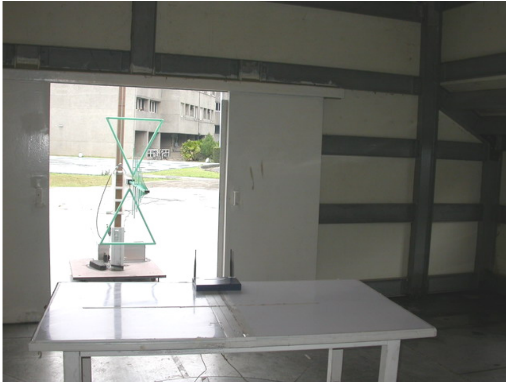
Antenna 1 (SNW0007A 1/2 \lambda Dipole 5dBi)
