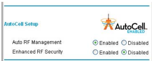
Figure 5-3: Advanced Wireless Settings screen AutoCell Setup options
