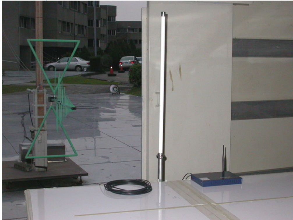
Antenna 4 (ANT24P12 GP Omni-directional 12dBi)
