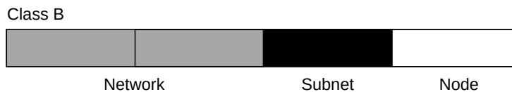
Figure B-2: Example of Subnetting a Class B Address
