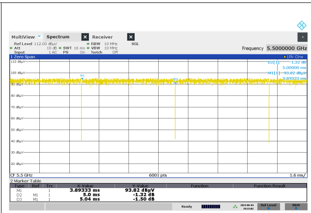
802.11be EHT20, OFDMA, 52T+26T, 2Tx
