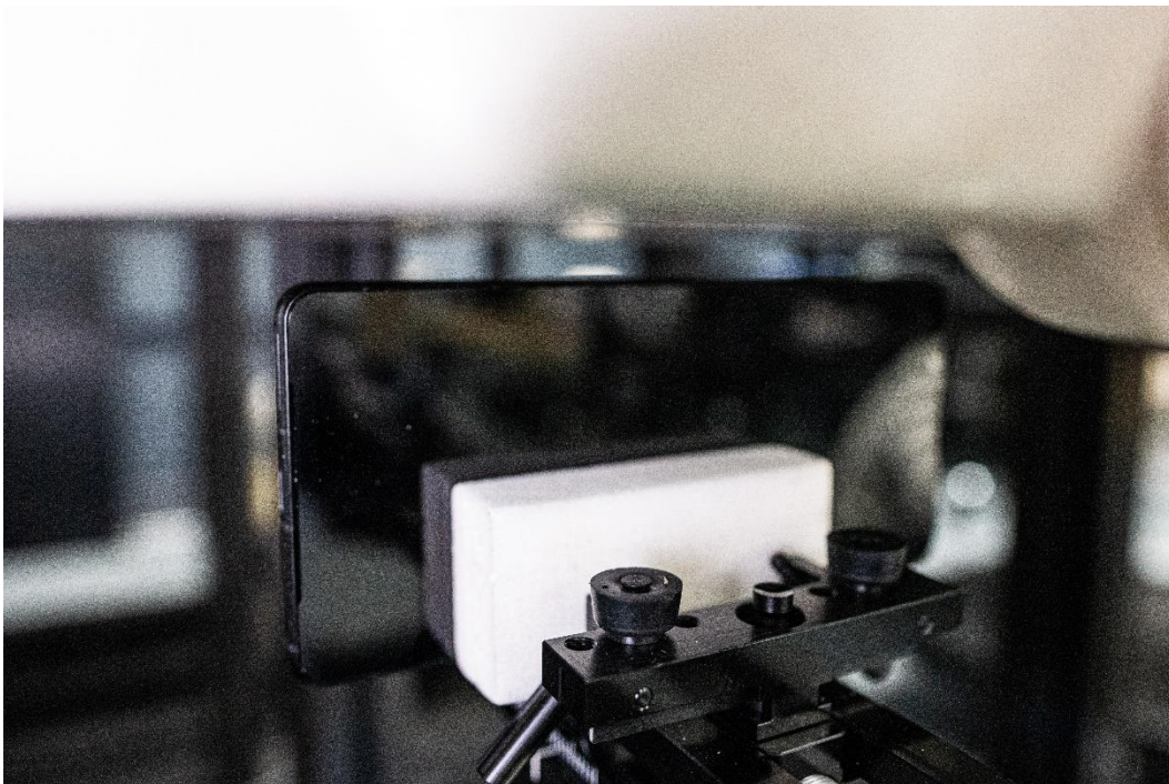
Figure O SAR Test Setup – Hotspot – Left 10mm
