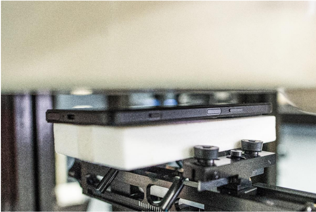
Figure H SAR Test Setup – Hotspot – Front 10mm
