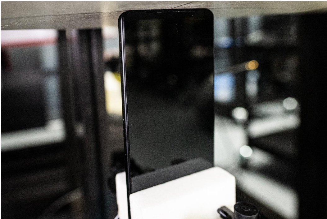
Figure M SAR Test Setup – Phablet – Bottom 0mm
