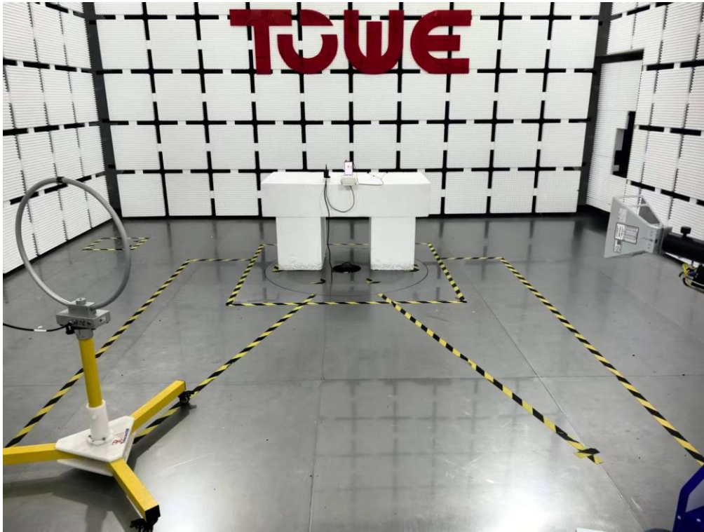
Radiated Spurious Emissions (9kHz to 30MHz)
