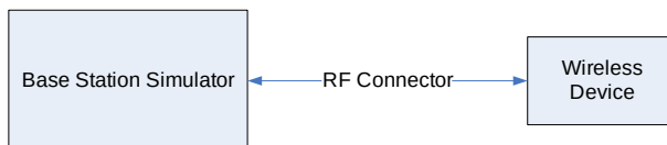
Figure 9-2 Power Measurement Setup
