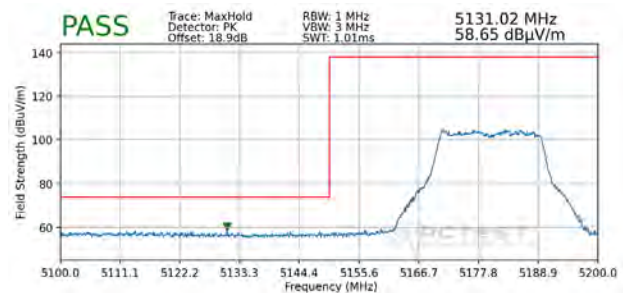
Plot 7-284. Radiated Lower Band Edge Plot SISO ANT1 (Peak - UNII Band 1)
