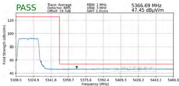
Plot 7-285. Radiated Upper Band Edge Plot SISO ANT1 (Average - UNII Band 2A)
