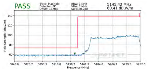
Plot 7-340. Radiated Lower Band Edge Plot MIMO (Peak – UNII Band 1)
