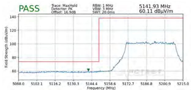
Plot 7-333. Radiated Lower Band Edge Plot MIMO (Peak – UNII Band 1)
