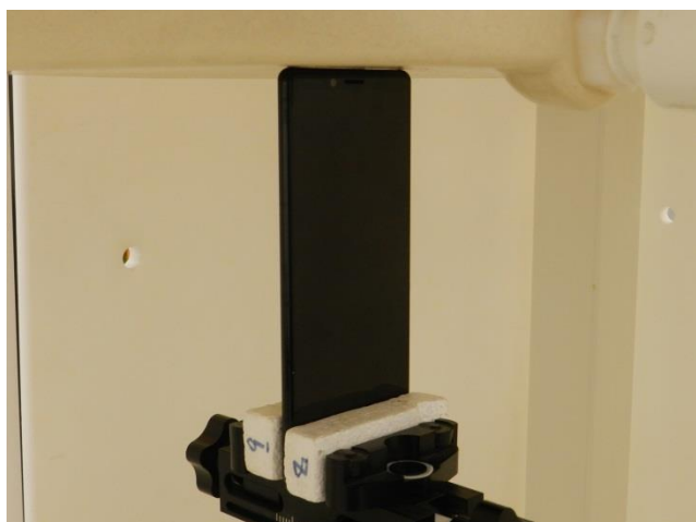
Top Side, Test Separation 0 mm
