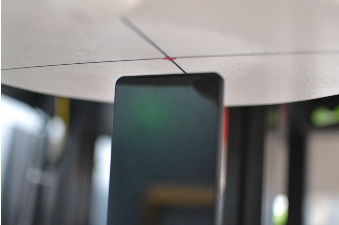
SAR Test Setup Photo 11 – Hotspot, Bottom Edge at 10mm
