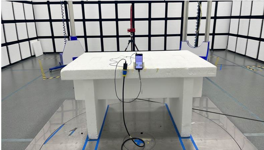
RADIATED PHOTO (0.009-30MHz NFC)
