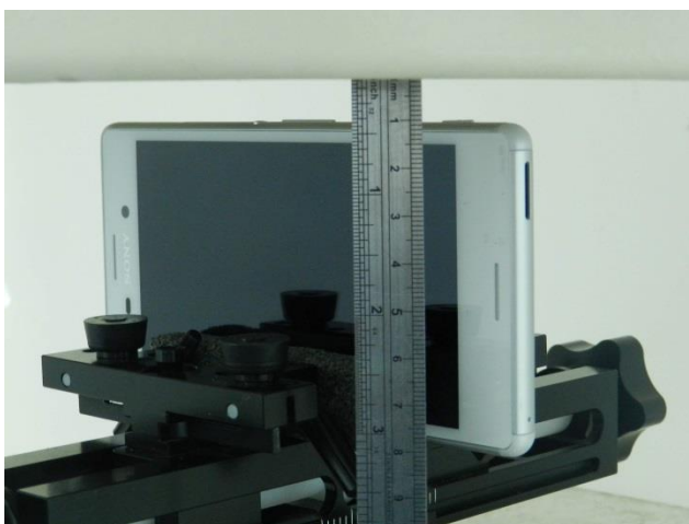
Right Side, Test Separation 1.0 cm
