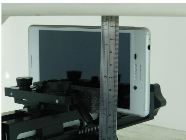
Left Side, Test Separation 1.0 cm
