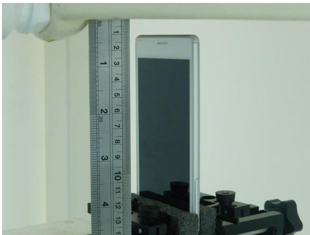
Bottom Side, Test Separation 1.0 cm
