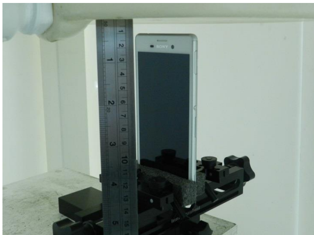
Top Side, Test Separation 1.0 cm
