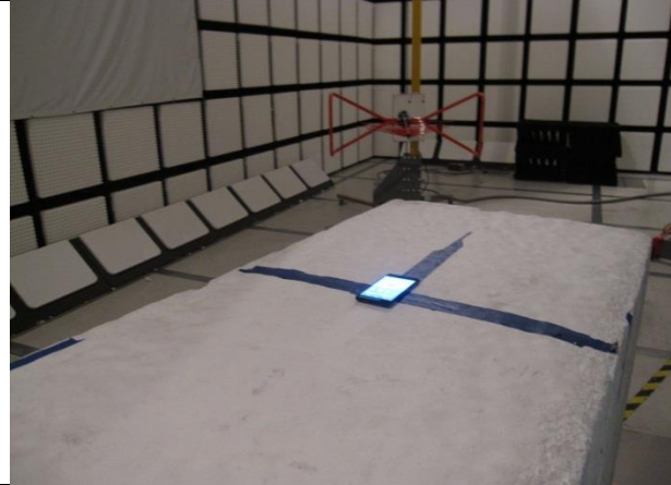
RADIATED FRONT PHOTO (BELOW 1 GHz)
