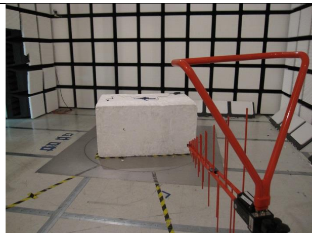
RADIATED FRONT PHOTO (BELOW 1 GHz)
