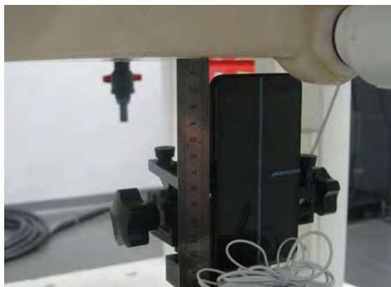
Fig.13 EUT bottom with headset to flat phantom
