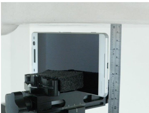
Right Side, Test Separation 10 mm
