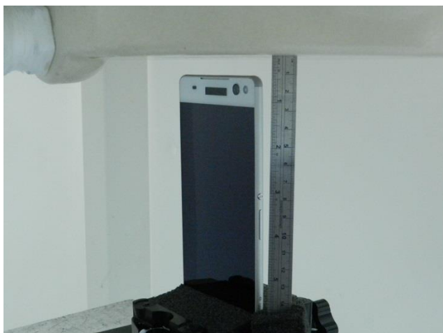
Top Side, Test Separation 10 mm
