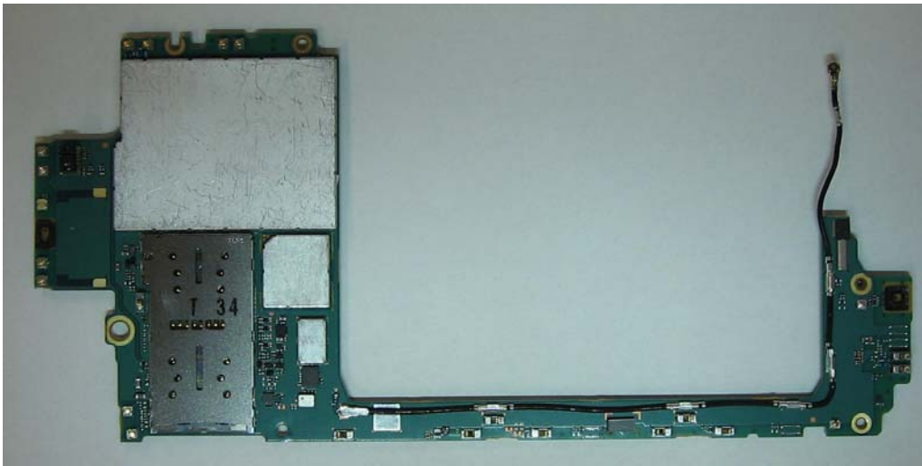
Internal PWB without Shield cases (Rear-side)
