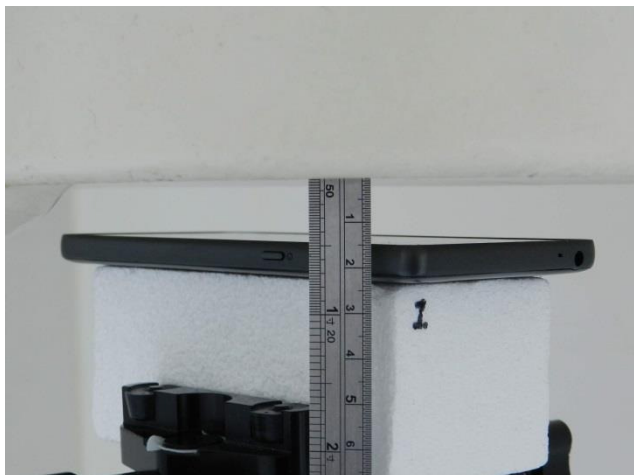
Front, Test Separation 15 mm
