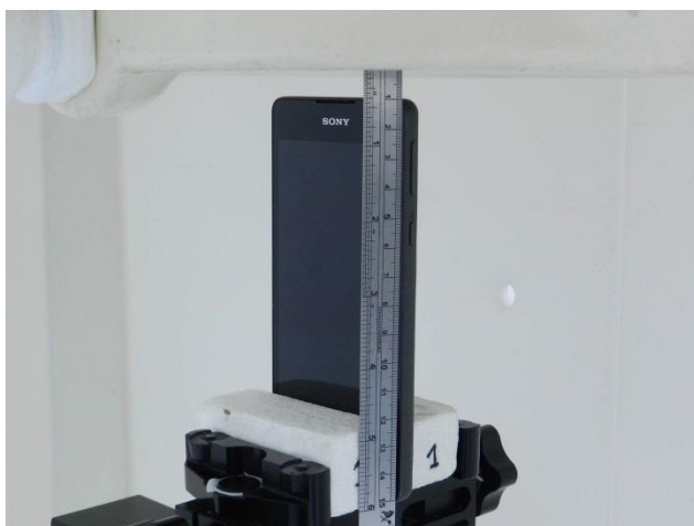
Top Side, Test Separation 10 mm
