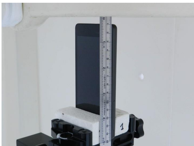
Bottom Side, Test Separation 10 mm
