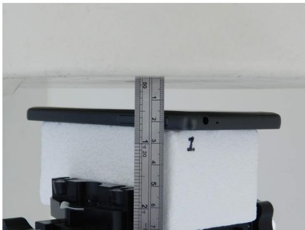
Back, Test Separation 15 mm
