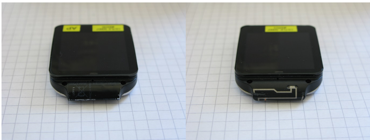
Illustration of the location of the WLAN/BT antenna (exposed on right)
