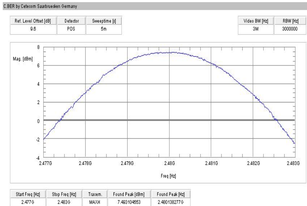
Plot 6: highest channel – 2480 MHz, Pi / DQPSK modulation
