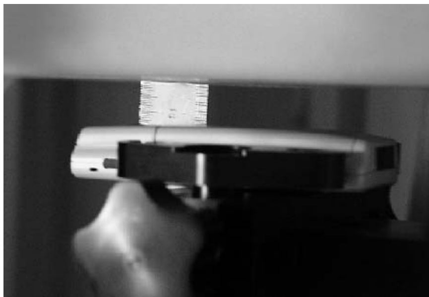
Device position against the body: Backside Phone holds 15cm away from the flat position of phantom
